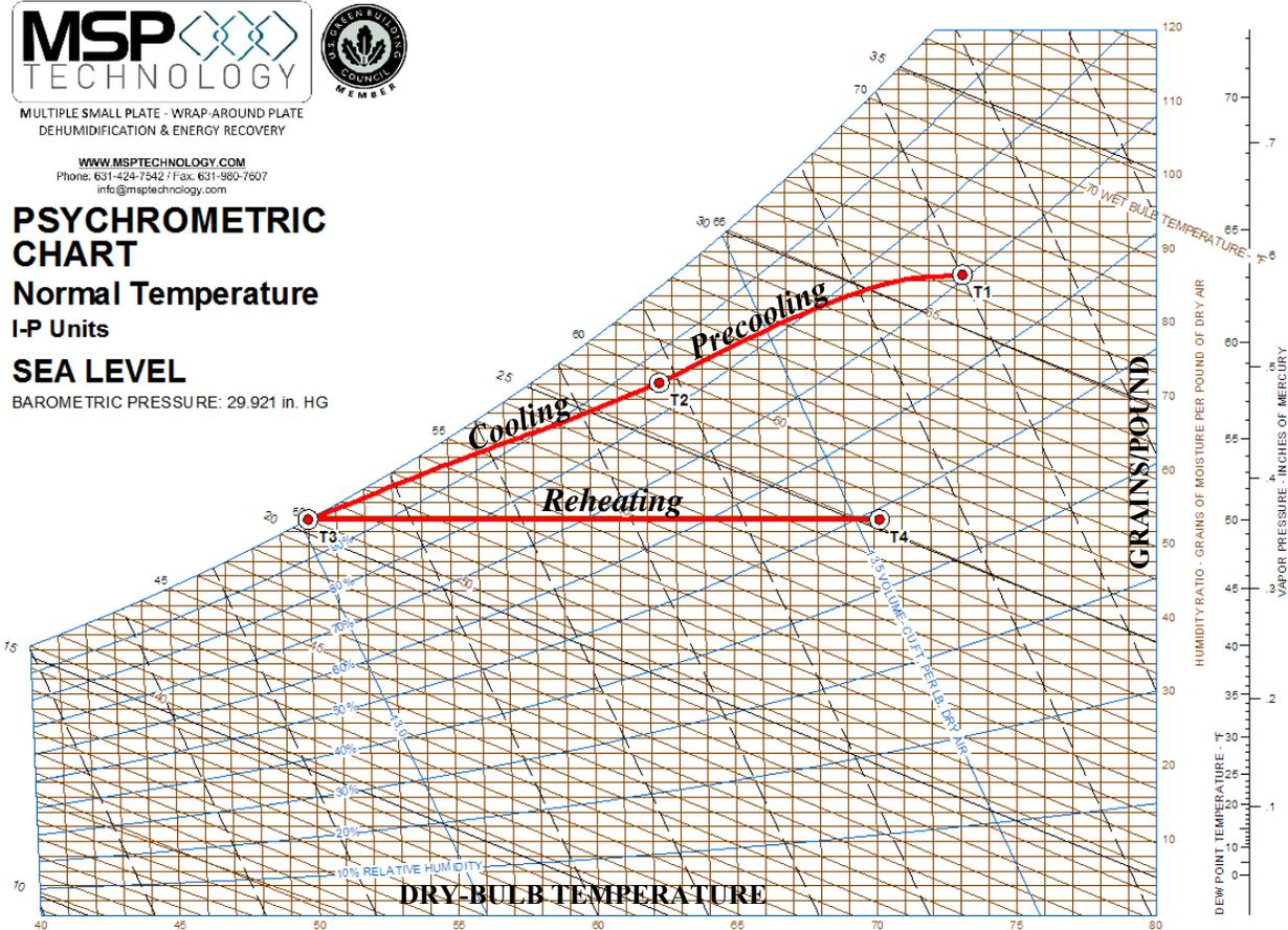
NOTE: Chart shows MSP DOAS profile. Conventional DOAS profile is similar. Outdoor air travels directly from T1 to T3, with no precooling and T3 to T4 is hot gas reheat.
