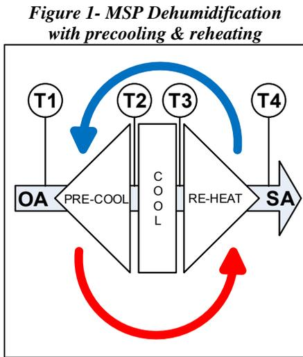
Wrap-around plate precools (T1-T2) Saving significant energy (T2-T3)
