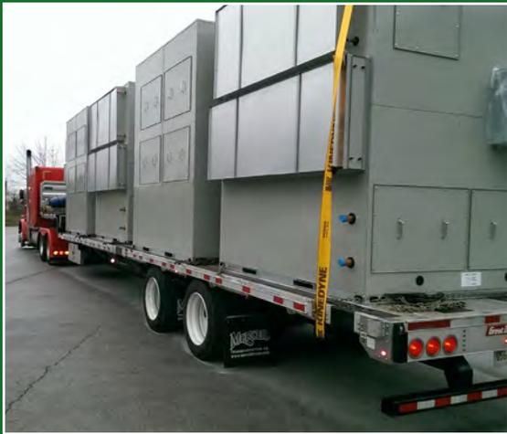
MSP Technology provided its dehumidification, climate control and water recovery solution for a grow facility in Massachusetts. It consists of 84,500 CFM of chilled water dehumidification and 200 tons of capacity serving multiple cultivation rooms.
